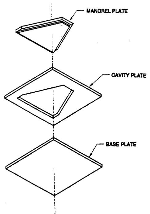
Figure 6. Equipment Tray Mold
