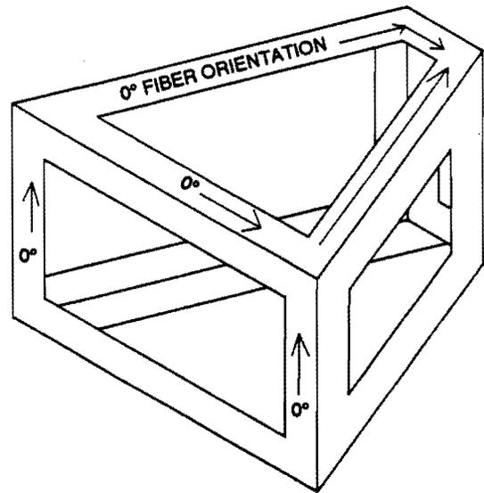
Figure 4. Frame Fiber Orientation
