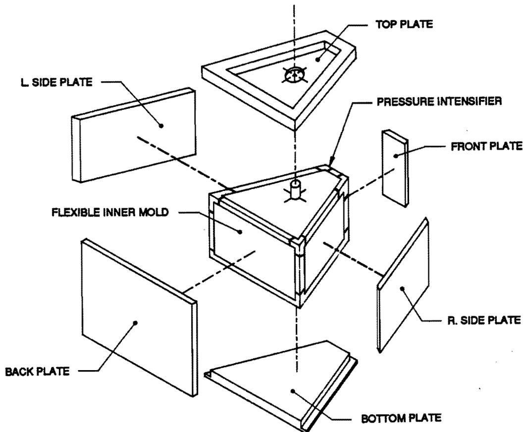
Figure 3. Frame Mold
