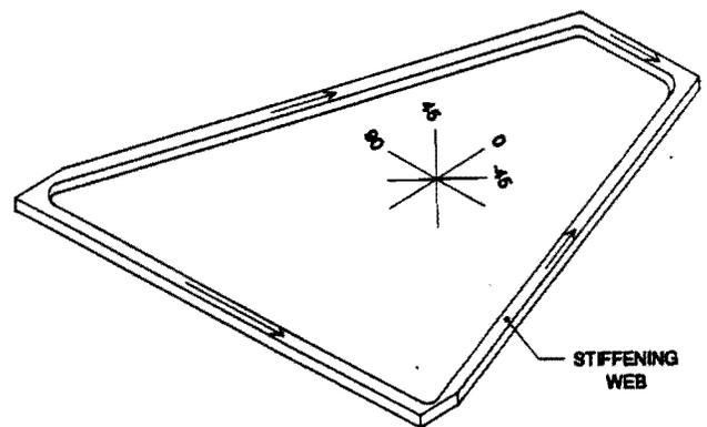
Figure 7. Equipment Tray Fiber Orientation
