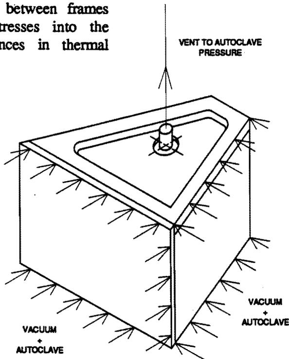
Figure 5. Frame Pressure Schematic
