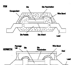
Figure 1. PEM vs. hermetic construction
