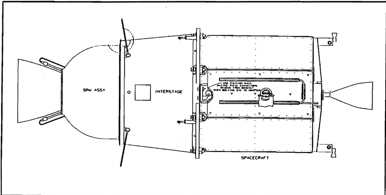
**Figure 1: Clementine Space Vehicle and Components**
