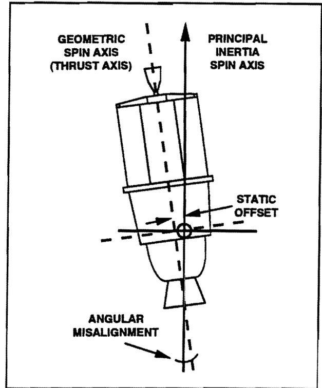
Figure 2: Clementine Space Vehicle Spin Axes Definition
