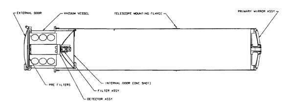
Figure 3. Layout of the SWATH high resolution X-ray instrument.
