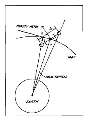
Figure 1. Spacecraft Axis System<sup>2</sup>
