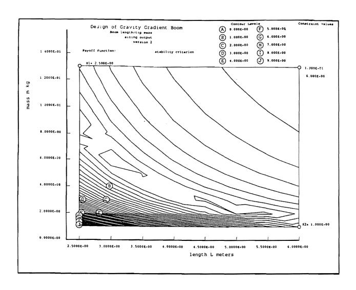
Figure 10. Boom Sizing Contour Plot
