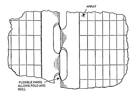
Figure 2.1.1-2. Array Hinge Design
