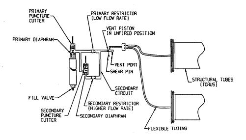
Figure 2.2.2-2. Inflation System Schematic
