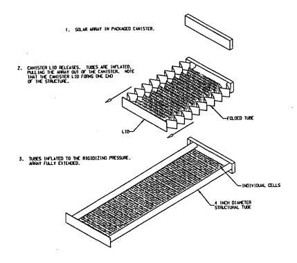
Figure 2.2.2-1. ITSAT PH2 Design
