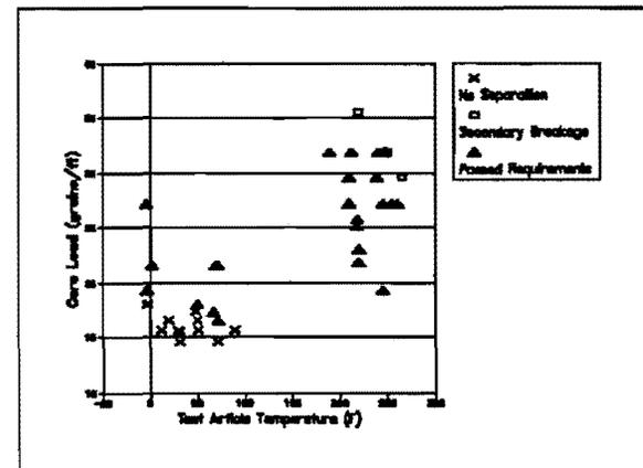
Determining the minimum core load required to reliably separate the aluminum extrusion and the maximum tolerated without secondary breakage were the objectives of this test approach. As Figure 9 shows, the separation threshold was approximately 18 grains/ft.
