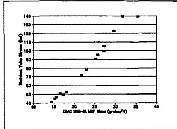
Figure 8 Stress in 0.049 inch Stainless Steel Tube
