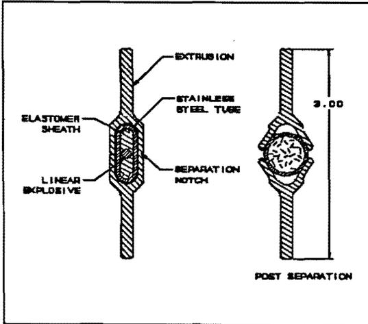
**Figure 4** Frangible Joint Before and After Function
