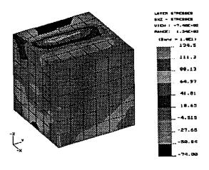
Fig. 6 Distribution of transverse shear stress in the core
