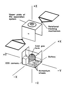
Fig. 2 SATEX-1 exploded view
