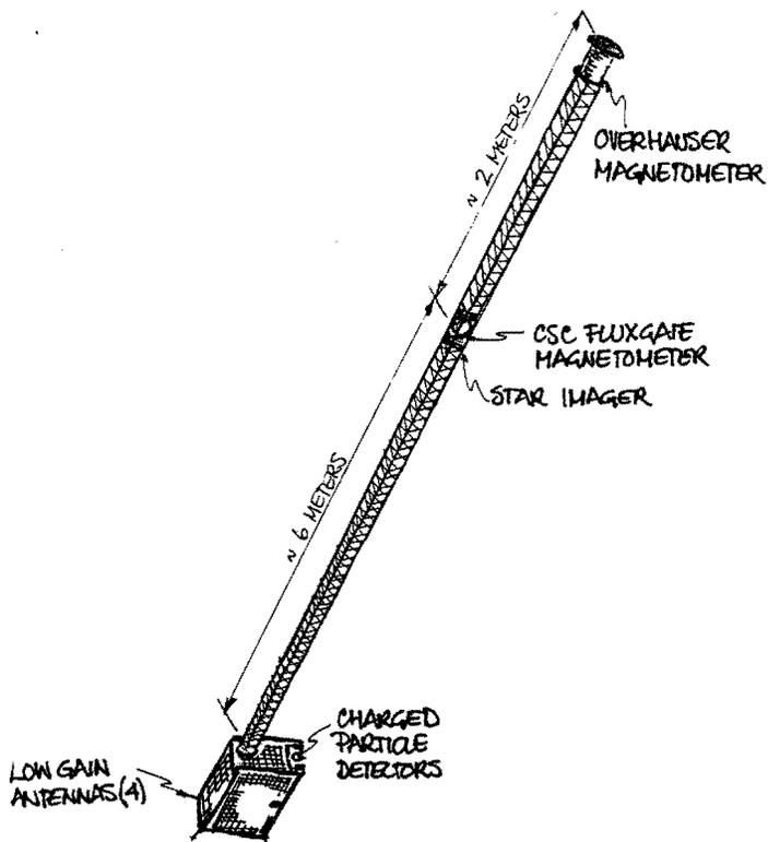
Figure 2: Ørsted Satellite in the Orbital Configuration
