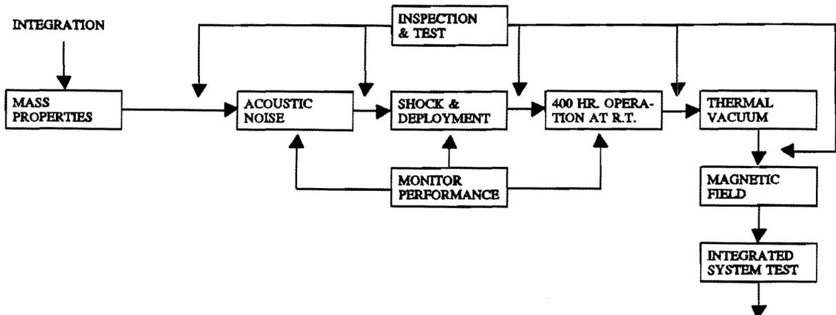
Figure 10: Satellite Acceptance Test Sequence
