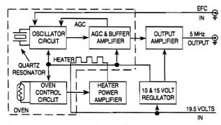
Figure 3. Ultrastable Quartz Oscillator Functional Block Diagram.
