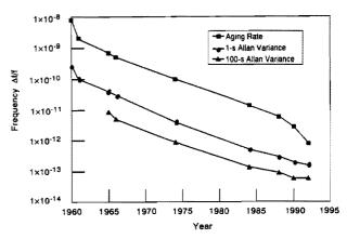
Figure 9. Frequency Stability History of APL Quartz Oscillators.
