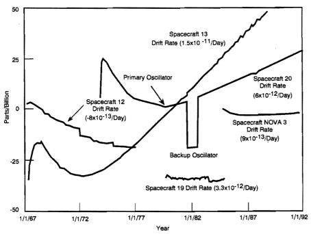
Figure 1. Oscillator Performance of NNSS Spacecraft.
