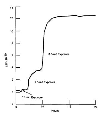
Figure 10. Frequency Response of Quartz Resonator SN33820 to Ionizing Radiation. Dose Rate = 0.1 rad (Si)/min.
