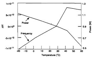
Figure 11. Oscillator Performance in a Vacuum Versus Temperature.
