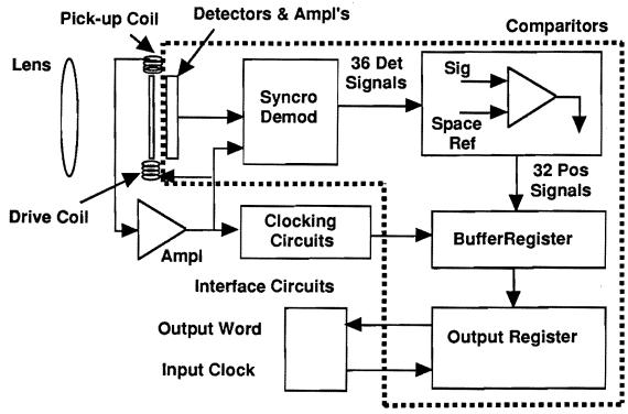
Figure 4, Low Accuracy Block Diagram
