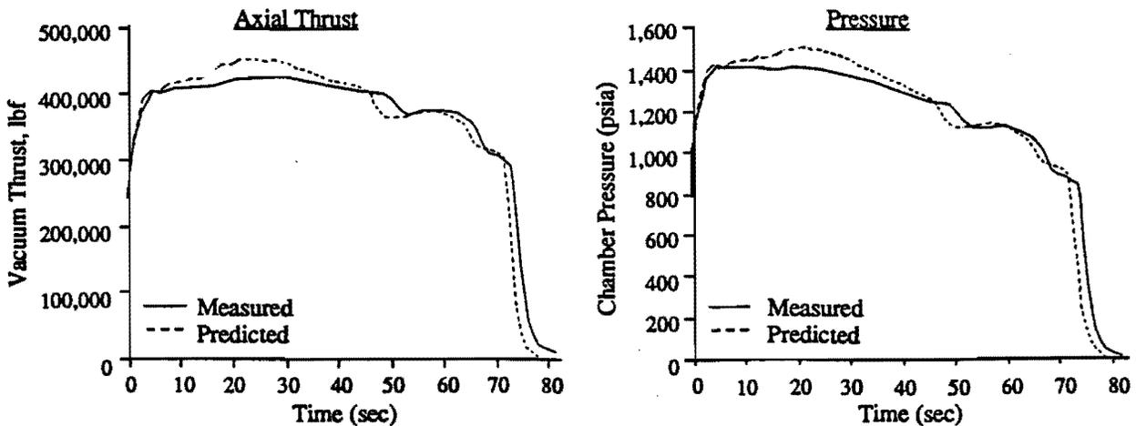
Figure 2. Castor 120™ Rocket Motor Performance
