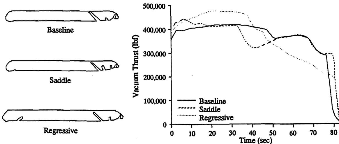
Figure 5. Castor 120™ Rocket Motor Performance Tailoring
