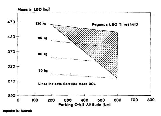
Fig. 7 Pegasus 4-stage GEO payload performance payload mass versus parking orbit altitude for an equatorial launch.
