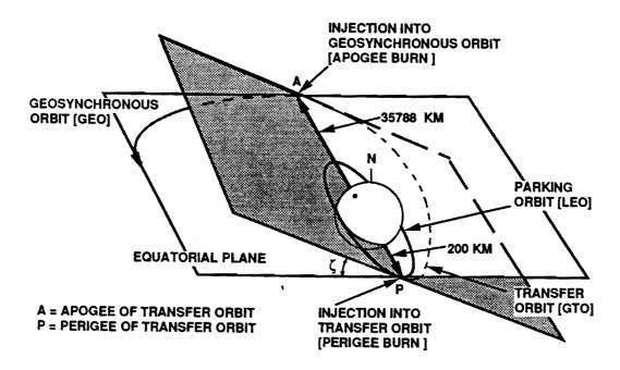
Fig. 2 Orbit parameters for Geosynchronous Launch Sequence
