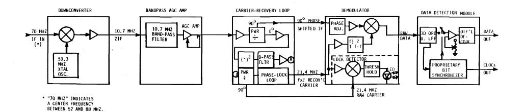
Figure 4. CMX9600 Modem Block Diagram
