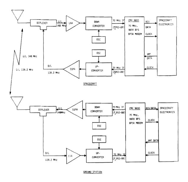
Fig. 3 Bremsat Communications System Block Diagram
