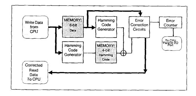
Fig. 1 Hamming Error Detection and Correction for the OBC Memory
