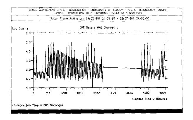
Fig 4. Solar-Flare Enhancements of the Auroral Oval Region Detected by the UoSAT-3 Cosmic Particle Experiment
