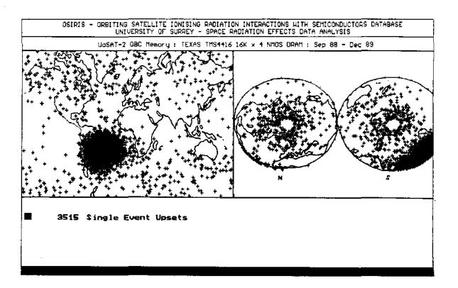
Fig. 2 UoSAT-2 OBC Memory SEU Activity Plotted Against Orbital Position
