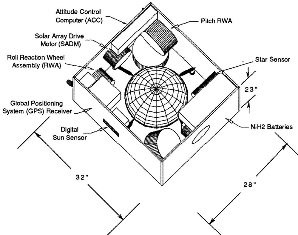
Figure 1. MPS Configuration.
