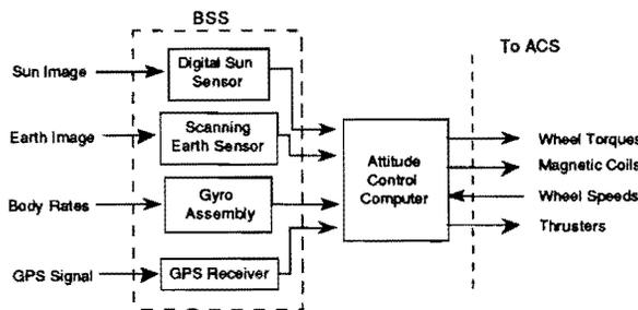
Figure 4. Functional Block Diagram of Basic Sensor Subsystem
