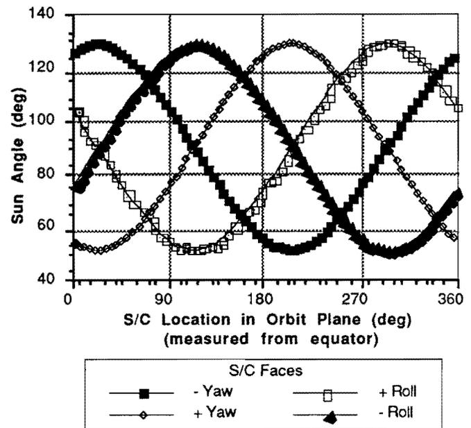
Figure 2. Sun Angle on Spacecraft Versus Orbital Position
