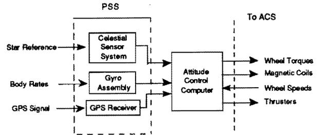
Figure 5. Functional Block Diagram of Basic Sensor Subsystem
