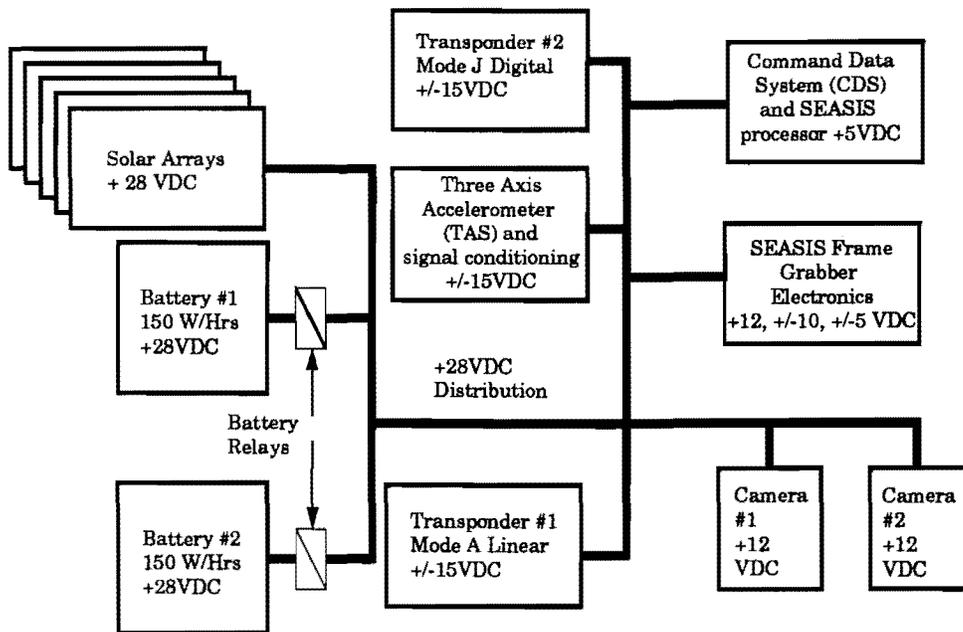
Figure 3 Electrical Power System Functional Block Diagram
