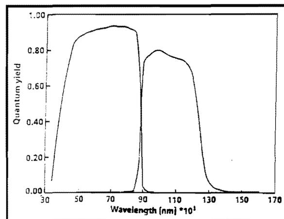
Figure 6 Spectral Response of A Tandem Cell
