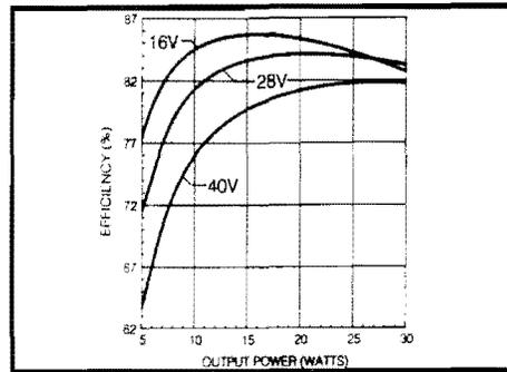
**Figure 7 SEDSAT 1 typical DC-DC converter efficiency**
