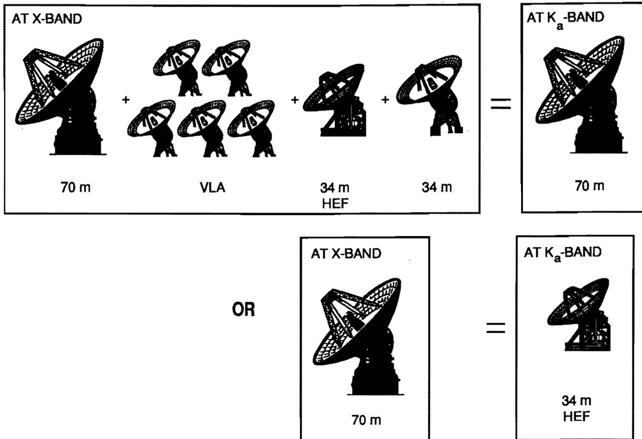
Figure 3. The X- and  $K_a$ -band G/T Equivalences
