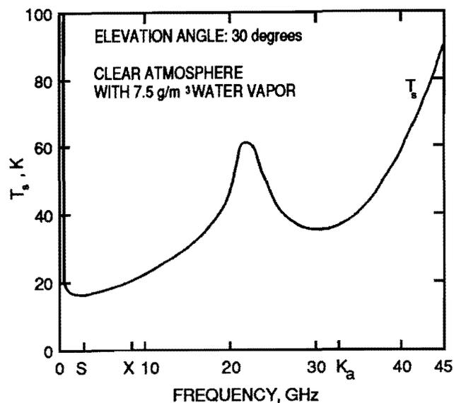
Figure 1. Projected DSN 70-meter antenna system temperature
