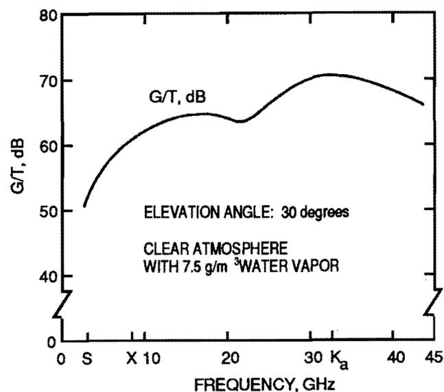
Figure 2. Projected DSN 70-meter antenna system Gain vs. System Temperature ( $G/T$ )
