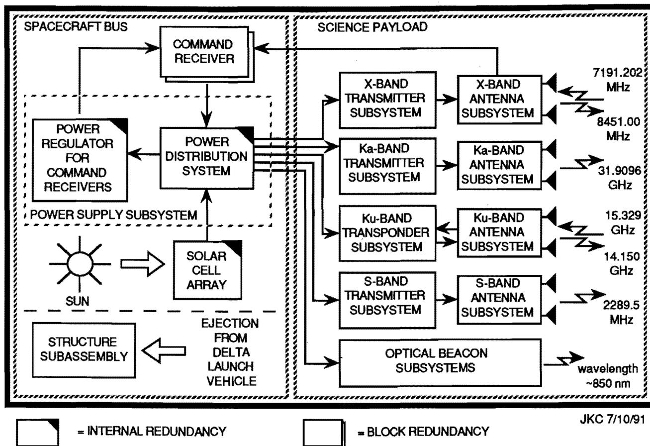
Figure 4. SURFSAT Functional Block Diagram
