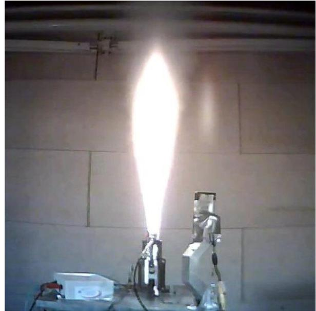
**Figure 5: NKS firing on thrust frame**
