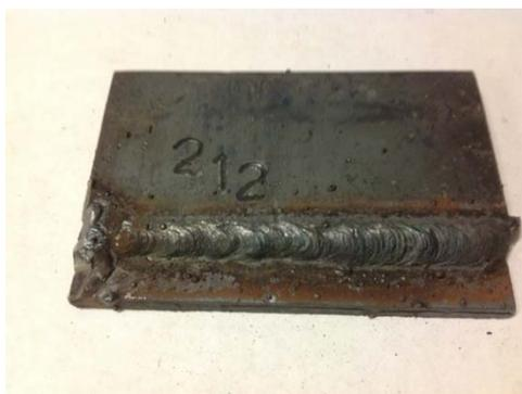
Figure 6. SMAW weld test coupon.
