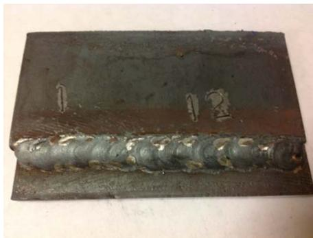
Figure 5. GMAW weld test coupon.
