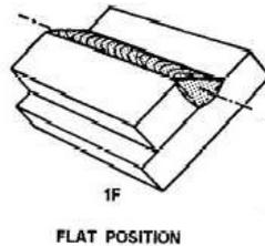
*Figure 1.* American Welding Society 1F (Flat-Horizontal) position.
