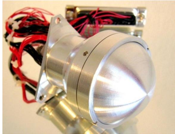
**Figure 14: PRISMA thruster module that accommodates four proportional milli-Newton MEMS thrusters.**
