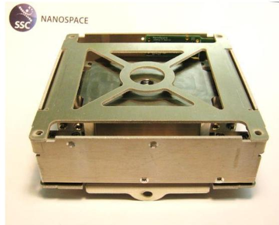
**Figure 1: First breadboard of the MEMS-based micro propulsion module comprising four closed-loop thruster controlled MEMS thrusters and a centralized Titanium tank in a 100x100x30 mm package.**
