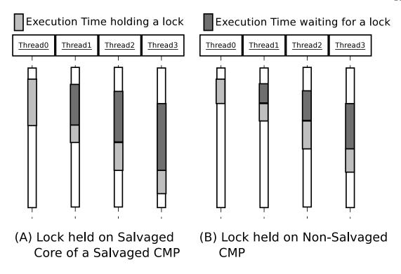
Fig. 4.1: A diagram showing how synchronization causes slowdown to propagate.
