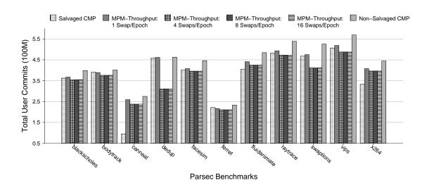
Fig. 7.7: A comparison of the number of swaps per epoch for the throughput balancing triggered variation.
