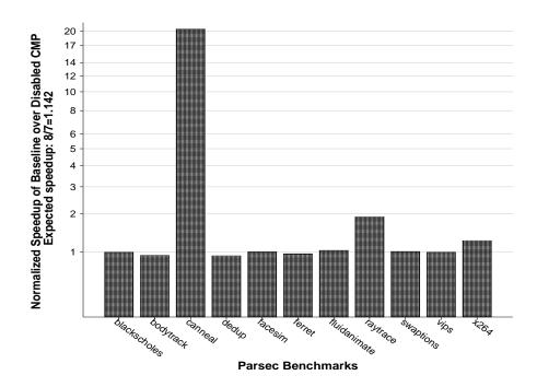
Fig. 2.1: A comparison of multi-threaded performance of a disabled CMP normalized to a non-salvaged CMP: The non-salvaged CMP is a homogeneous eight-core CMP, while the disabled CMP is a seven-core CMP.
