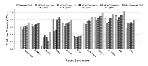
Fig. 7.4: A comparison of different the epoch length values for the throughput balancing triggered variation.
