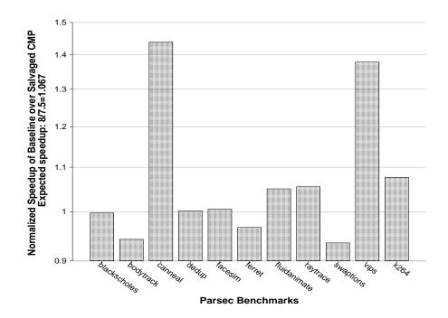
Fig. 2.2: A comparison of multi-threaded performance of a salvaged CMP normalized to a non-salvaged CMP: The non-salvaged CMP is a homogeneous eight-core CMP, while the salvaged CMP is a heterogeneous eight-core CMP with one half-speed core.
