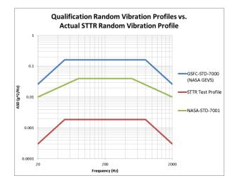
Figure 10: Random vibration test profiles.
