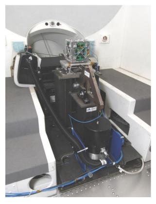
Figure 11: Picture of the test fixture installed onto the centrifuge, including the DUT (CubeSat satellite)
