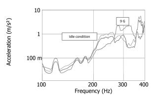
FIGURE 17: Z AXIS SINE SWEEP RESPONSE AT 9G FOR TRANSVERSE TEST FIXTURE. GREEN LINES REPRESENT TARE SWEEPS AT 1.4G.
