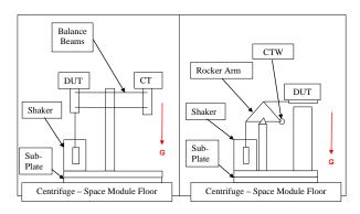
Figure 4: Parallel Fixture (left), Transverse Fixture (right). Red arrow shows direction of G load.
