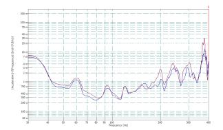
FIGURE 14: Y AXIS SINE SWEEP RESPONSE AT CENTRIFUGE IDLE (1.4G) BEFORE 3G, AFTER 9G TEST.
