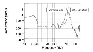
FIGURE 16: SIDE PANEL SINE SWEEP RESPONSE AT THE START AND END OF THE TESTING (BEFORE 3G, AFTER 9G) UNDER IDLE (1.4G) CONDITION.
