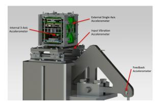
Figure 9: Internal 3-Axis Accelerometer and Single Axis Accelerometer Locations on Transverse Test Fixture.
