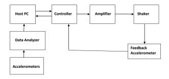
Figure 8: Closed loop connections between the PC, Controller, Amplifier, Shaker and Force Transducer.
