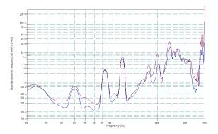
FIGURE 15: X AXIS SINE SWEEP RESPONSE AT CENTRIFUGE IDLE (1.4G) BEFORE 3G, AFTER 9G TEST.
