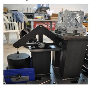
Figure 5: Transverse mode test fixture. Cylinder on the left is the shaker, and the square box on the right is the payload (CubeSat test pod)
