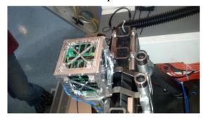
Figure 7: Close up of DUT installed on the parallel test fixture in Space Module.
