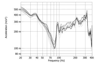
FIGURE 12: VIBRATION INPUT INTO THE DUT FOR THE TRANSVERSE FIXTURE.
