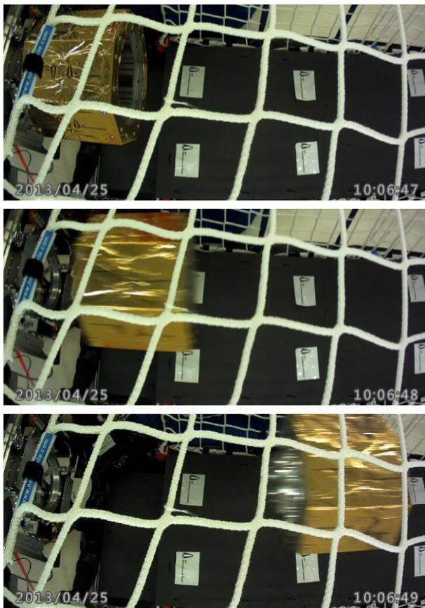
**Figure 4: Separation of Dummy Satellite during Parabolic Flight Campaign**
