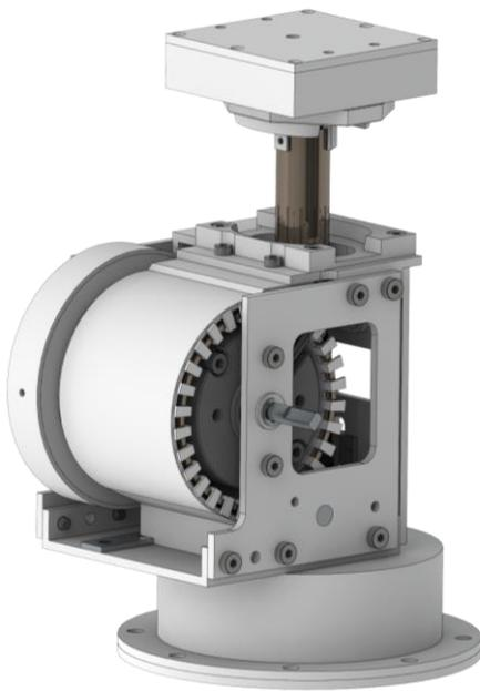
**Figure 7: CAD Model of the EBS assembly**
