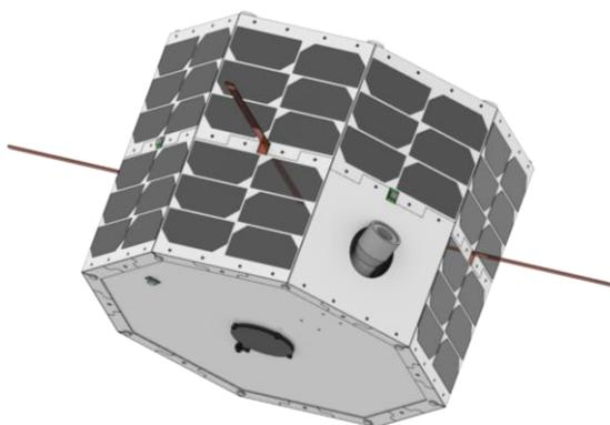
Figure 1: CAD Model of the TechnoSat Satellite
