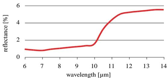
**Figure 6: Hemispherical Reflectance of the Metal Velvet Coating**
