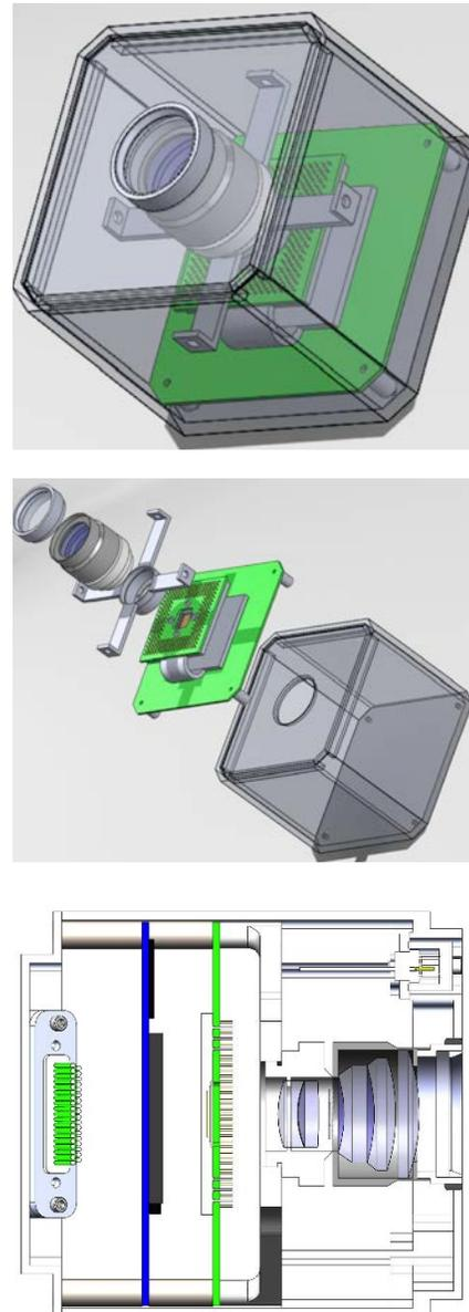
**Figure 5.** CAD of GRIFEX optical payload with camera, ROIC, and MARINA backend electronics.
