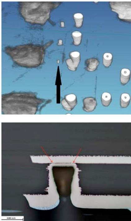
**Figure 3.** Microvia separation in SC-Mini board shown by computer tomography (top) and PCB board slicing (bottom).
