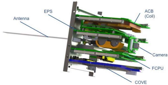
**Figure 1:** M-Cubed/COVE-2 and avionic redesign for launch and integration.
