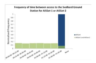
Figure 3: Distribution of the normalised frequency of revisit time to the Svalbard ground station for any of the AISSat satellites. The first bin indicates that both satellites are within ground station range within 0 – 15 minutes of each other. The bins increase in steps of 15 minutes up to 1 hour 30 min – 1 hour 45 min as a maximum.
