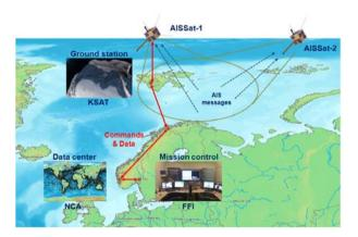
Figure 1: AISSat-1 mission architecture.
