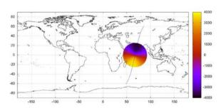
Figure 9: Induced Doppler shift (Hz) over the field of view of AISSat-1
