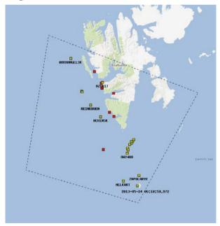
Figure 14: Multi hypothesis tracker output from satellite SAR imagery (dotted rectangle) fusion with Vessel Monitoring System (VMS), Long Range Identification and Tracking (LRIT) and AISSat-1 data. Red targets are unidentified SAR vessel detections, green targets are VMS, LRIT or AISSat-1 identified SAR detections.
