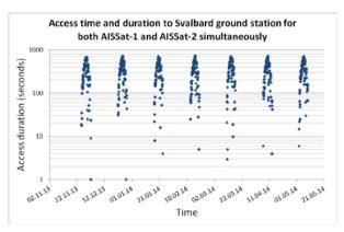
Figure 4: Access times and duration, in seconds, for both AISSat satellites contact with Svalbard.
