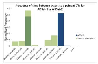
Figure 6: Distribution of normalised frequency of revisit time to a point at the equator for any of the AISSat satellites. The first bin indicates that both satellites are within view of the same point at the equator within 0 – 30 minutes of each other, while the second bin is for access within 30 min – 1 hour. The third bin indicates access within 1 – 2 hours, while the remaining bins then increase in steps of 2 hours up to 12–14 hours as a maximum.
