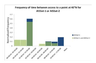
Figure 5: Distribution of normalised frequency of revisit time to a point at  $40^{\circ}N$  for any of the AISSat satellites. The first bin indicates that both satellites are within view of the same point at  $40^{\circ}N$  within 0-30 minutes of each other, while the second bin is for access within 30 min -1 hour. The third bin indicates access within 1-2 hours, while the remaining bins then increase in steps of 2 hours up to 10-12 hours as a maximum.
