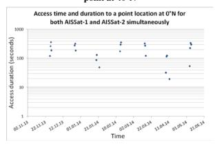
Figure 8: Access times and duration, in seconds, for simultaneous AISSat-1 and AISSat-2 contact with a point at 0°N
