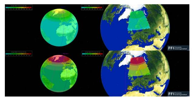
Figure 2: Average number of accesses per day globally (left) and in the area of interest (right) for AISSat-1 (top) and both AISSats combined (bottom). On the left hand side plots the colours run from 2 – 20+ in steps of 2, but on the right hand side the colours run from 7 to 28+ in steps of 3.
