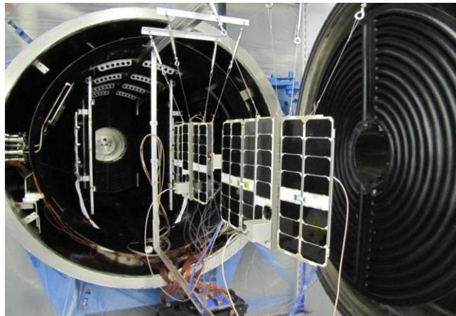
**Figure 2: SENSE Thermal Vacuum Test**
