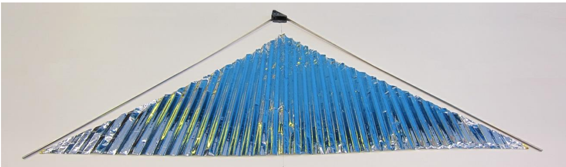
Figure 14: Drag Sail Qualification Model - Deployed
