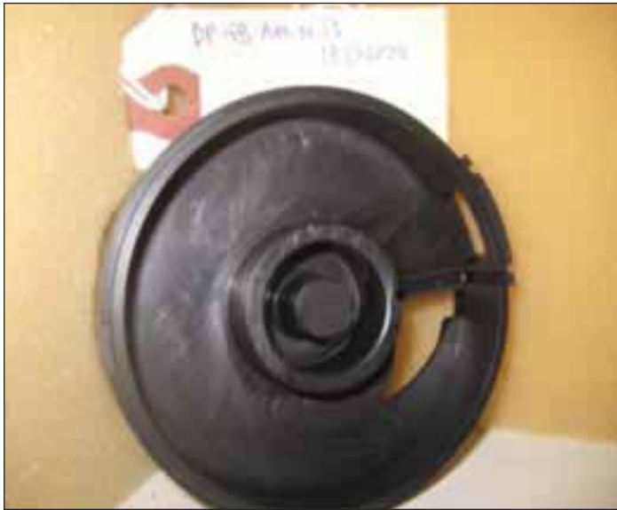
A displacement piston used in this study shows evidence of meter chamber scarring resulting from quartzite sand. This type of wear is not typically detrimental to the accuracy of the meter.
