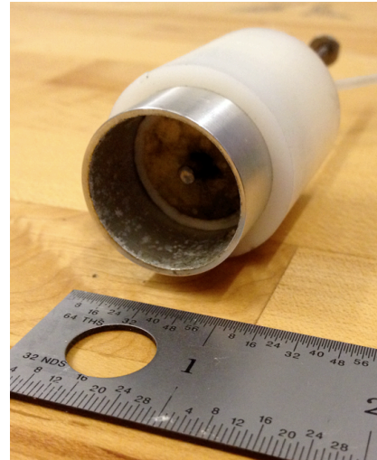
Figure 9: The coaxial PPT tested in this study.
