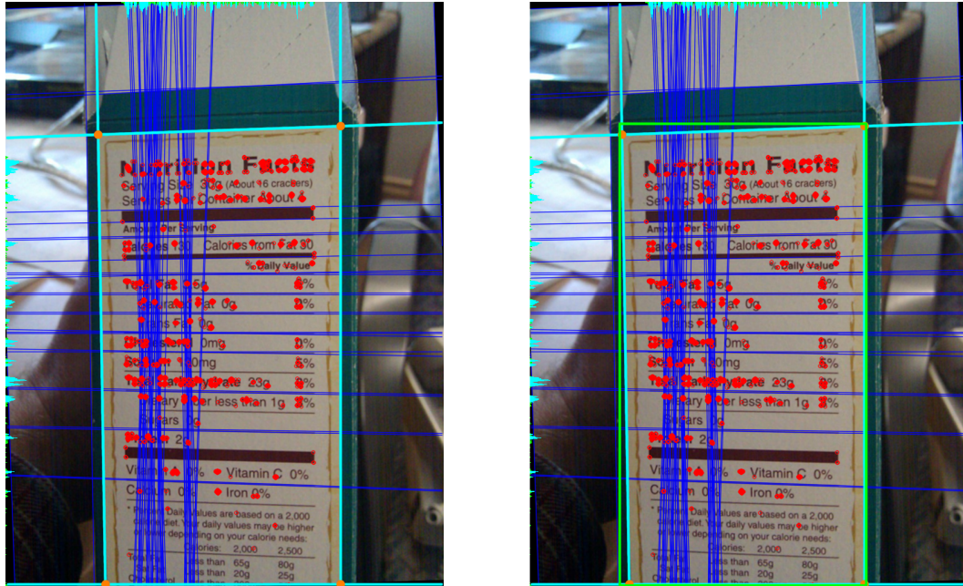
Figure 4.8. Simplification of Hough Boundary Lines
