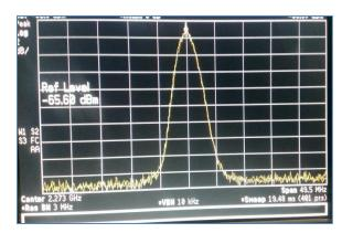
Figure 4: Spectrum Analyzer view of PULSAR S-Band signal.
