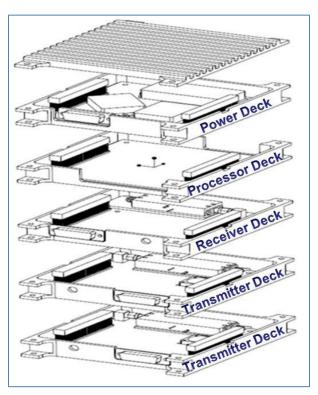
Figure 1: PULSAR contains five main component decks.
