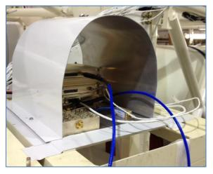
Figure 3: PULSAR with solar shield.
