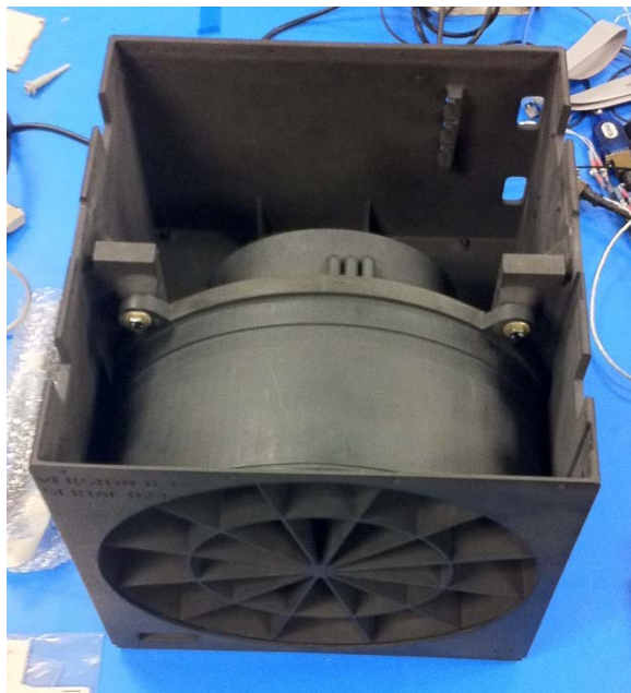
Figure 7: The ALTAIR™ Spacecraft 3-D printed structure.
