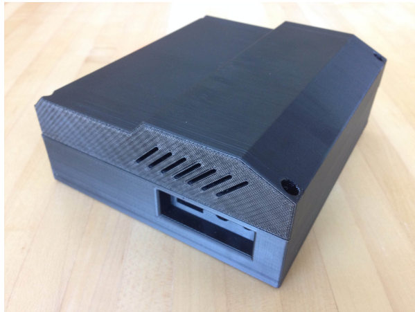
Figure 2: Rapid prototype of IMU enclosure
