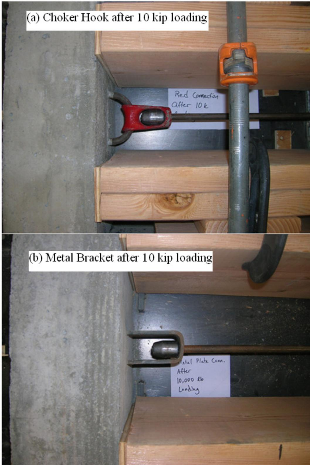
**Fig. 5.98.** Choker Hook (a) and Metal Bracket (b) connections after 10 kips loading
