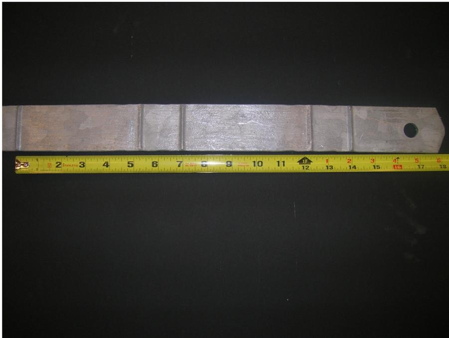
**Fig.4.77.** The RECO Strap bar
