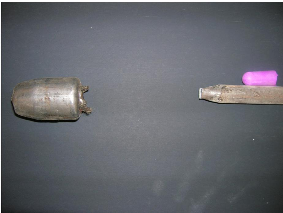
**Fig. 5.106.** Red Choker Hook connection failure at 15.1 kips
