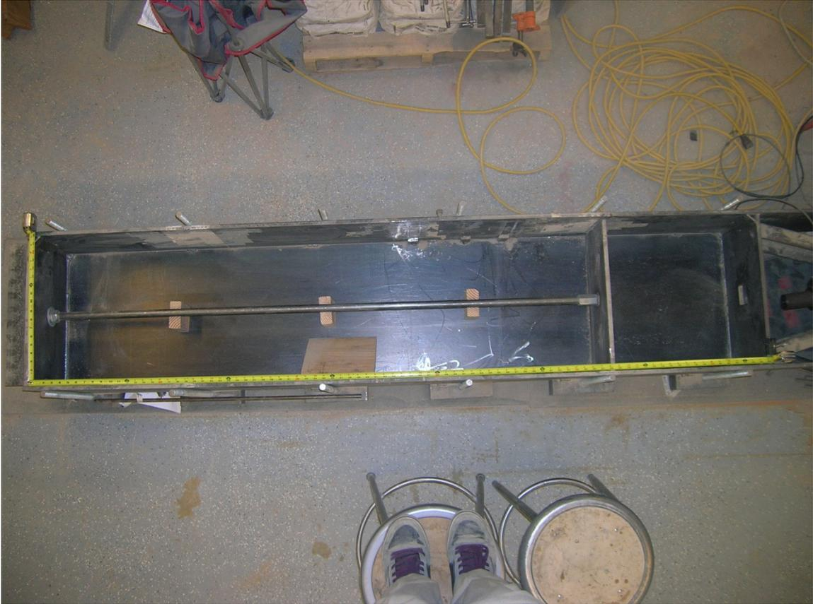
**Fig. 3.27.** Pullout box modification for crimp pullout tests
