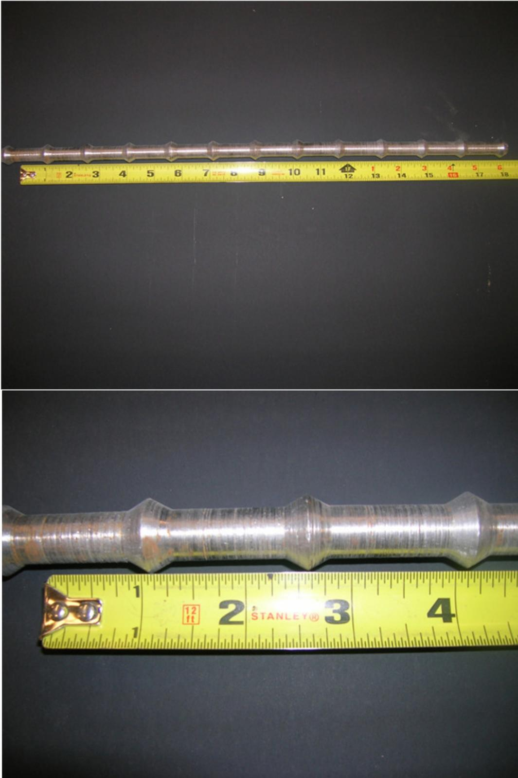
Fig. 4.62. 0.5 in. diameter bar with 30° taper
