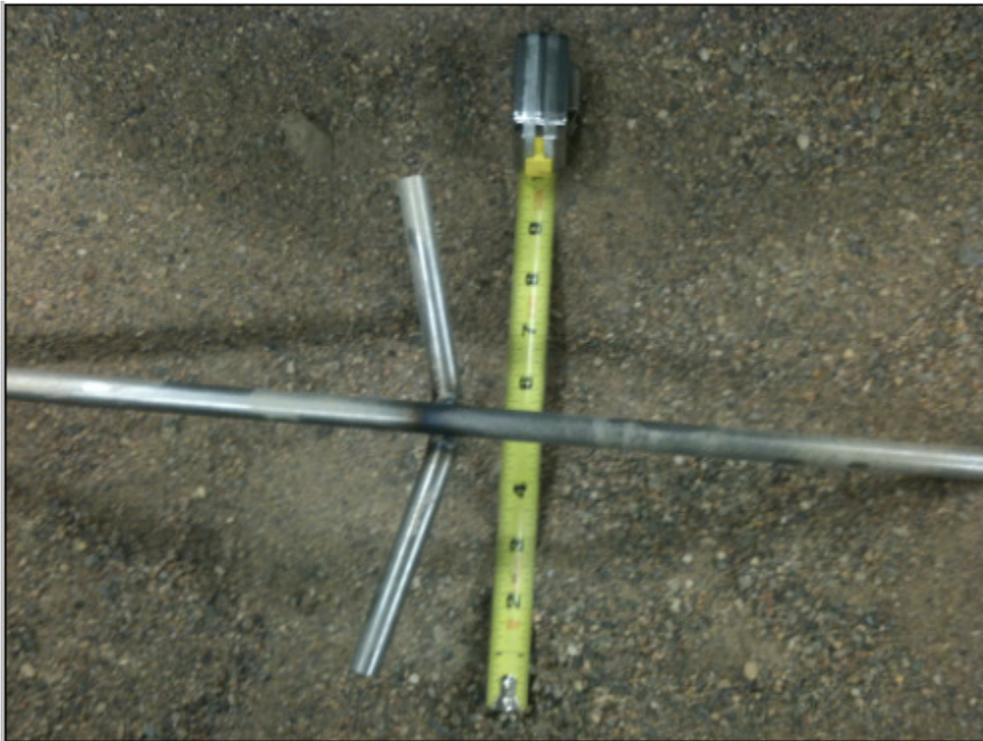
**Fig. 4.57.** 0.5 in. diameter cross bar with 8 in. length bent from the pullout test
