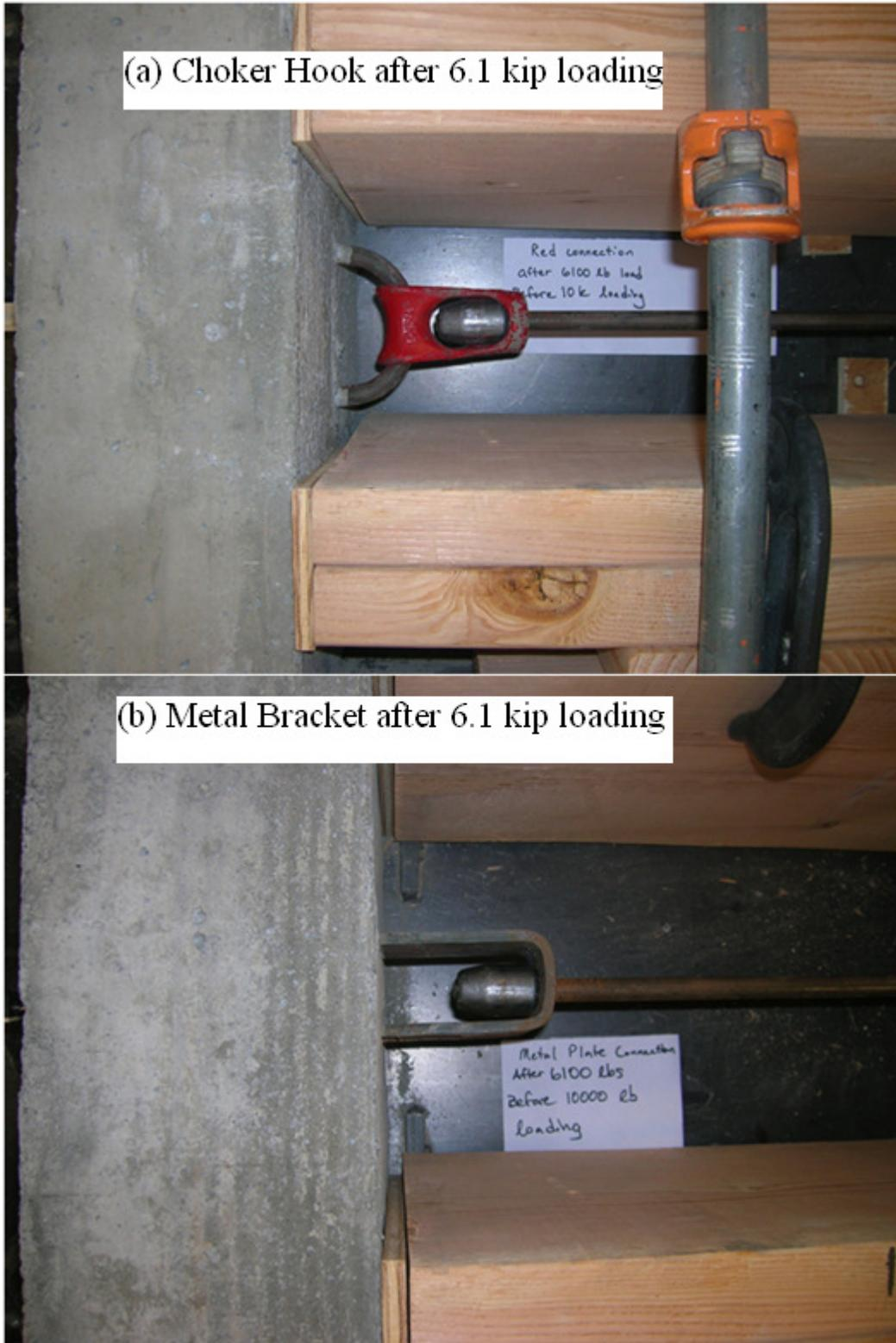
**Fig. 5.97.** Choker Hook (a) and Metal Bracket (b) connections after 6.1 kip loading and before 10 kip loading
