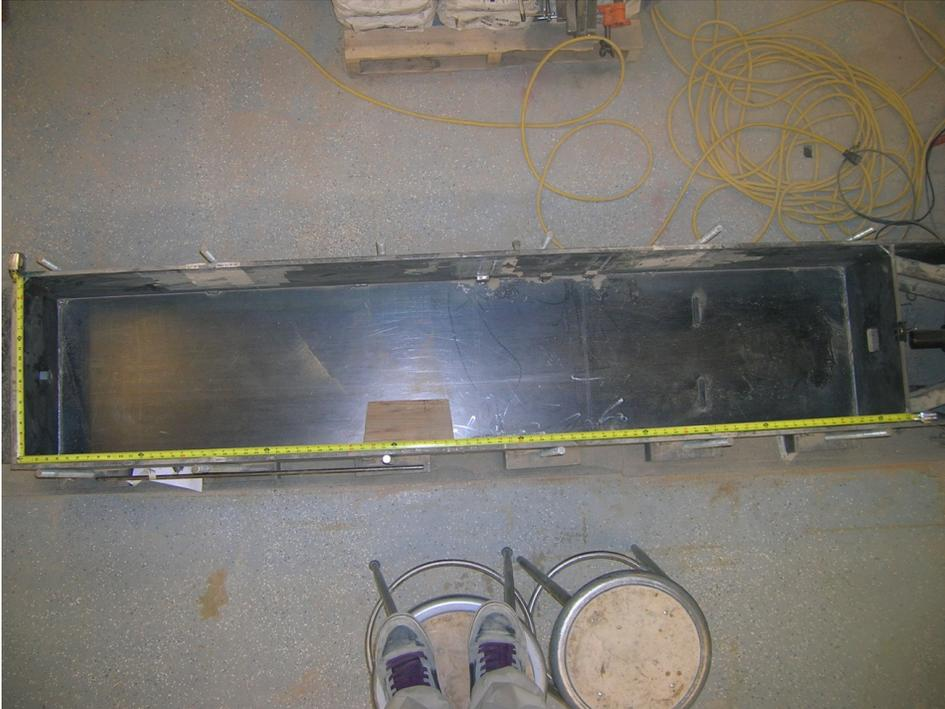
**Fig. 4.42.** Pullout box showing dimensions of 18 in. by 87 in.
