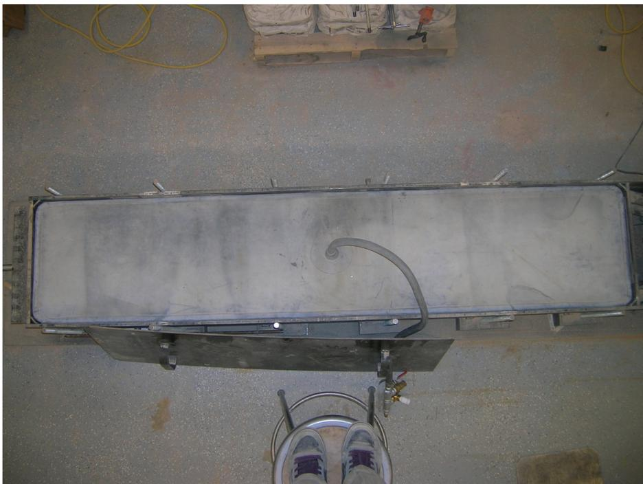
**Fig. 4.51.** Air bladder is placed on the lifts of sand after compaction
