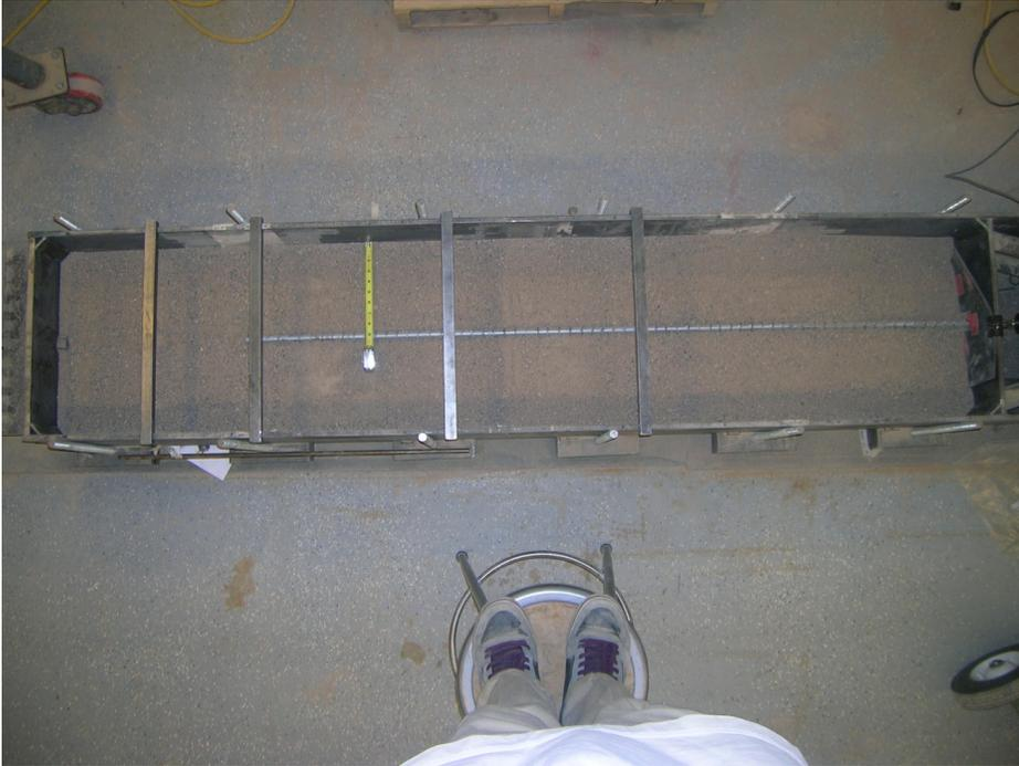
**Fig. 4.48.** Top view of pullout box after compaction of first lift
