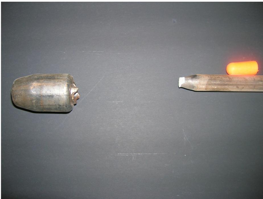
**Fig. 5.105.** Metal Bracket connection failure at 16.4 kips
