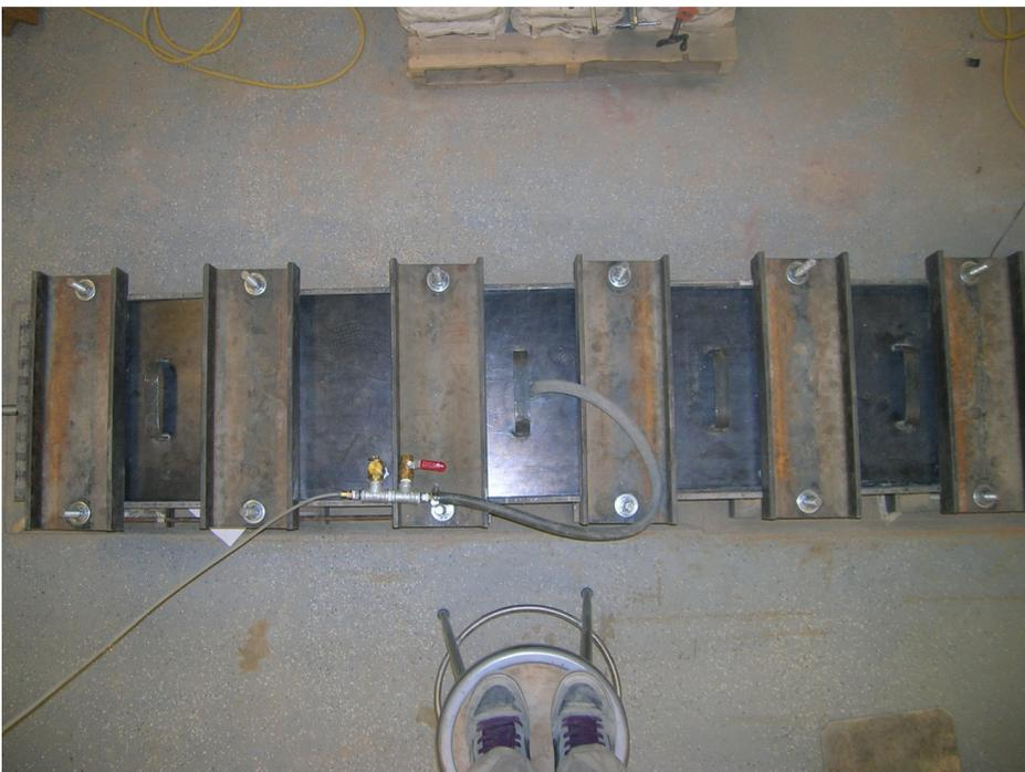
**Fig. 4.53.** The pullout box is ready for testing
