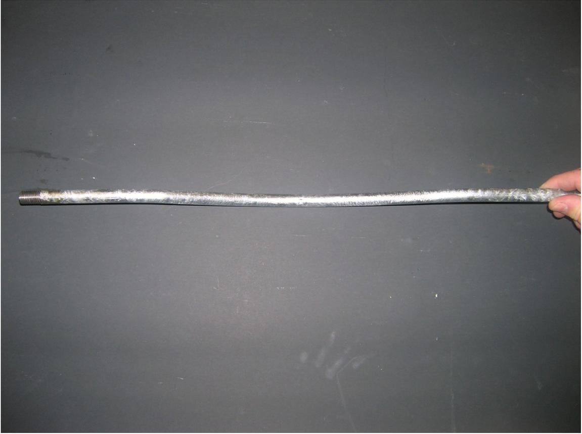
**Fig. 6.114.** 2.0 in. galvanized crimp
