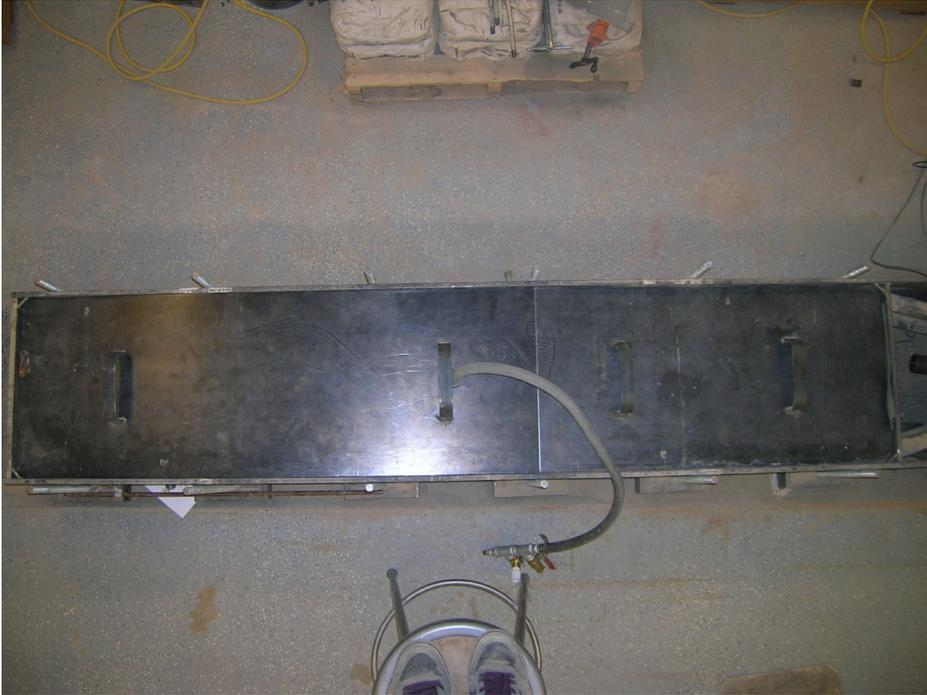
**Fig. 4.52.** The pullout box lid is placed on top of the bladder
