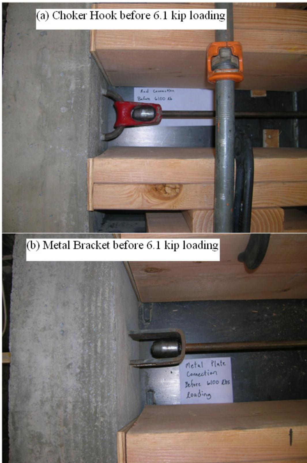
**Fig. 5.96.** Choker Hook (a) and Metal Bracket (b) connections before 6.1 kip loading
