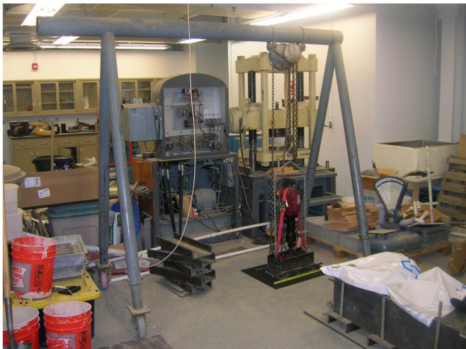
**Fig. 4.44.** Rolling lift structure with pulley and compacter and compaction foot
