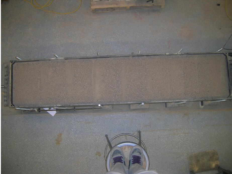
**Fig. 4.50.** Pullout box after second lift is compacted
