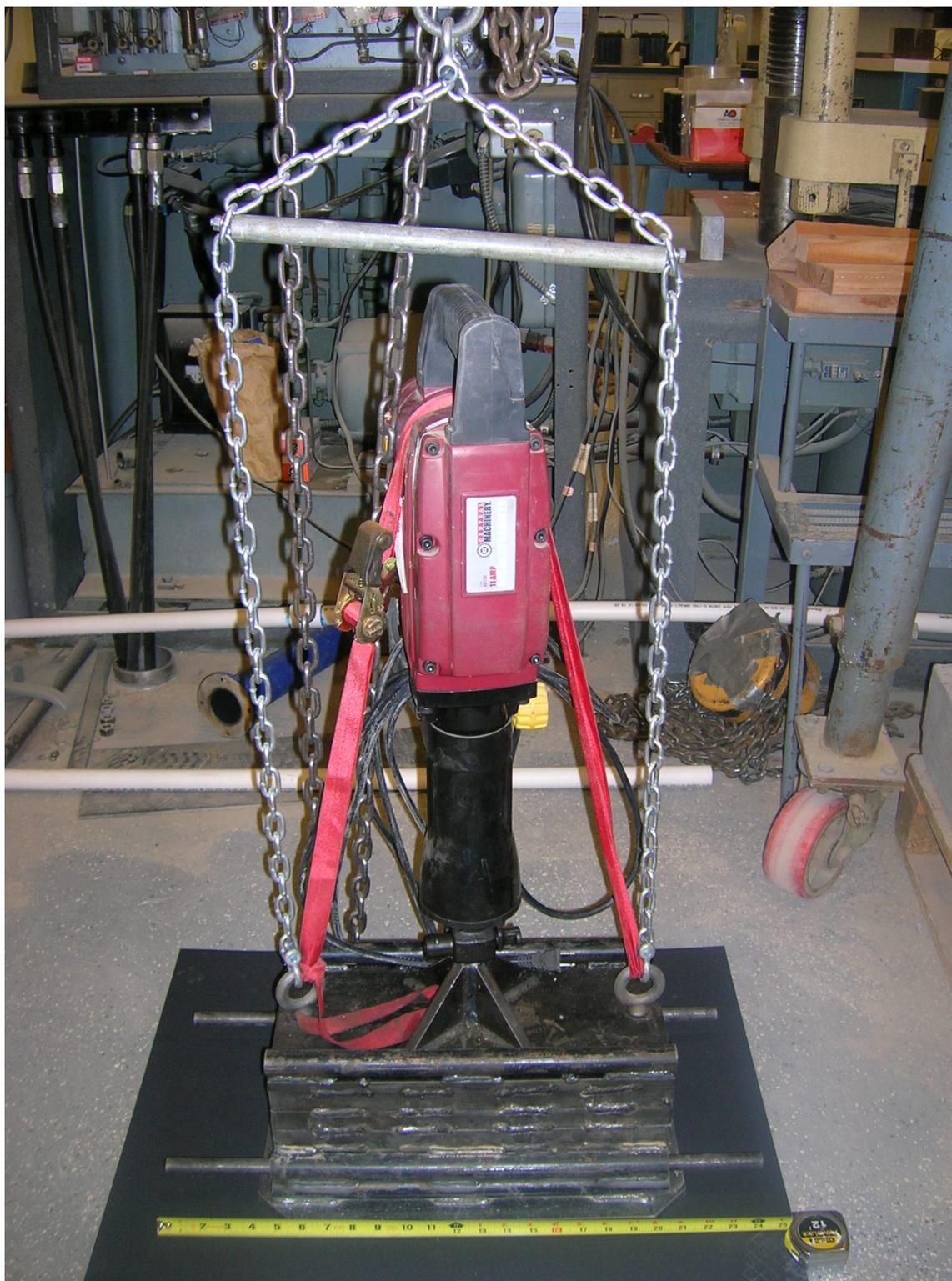
**Fig. 4.41.** Close up of compactor and compaction foot
