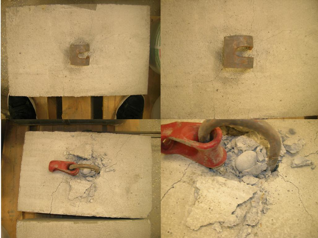
**Fig. 5.103.** Concrete connections after test using the Tenius and Olsen machine.
