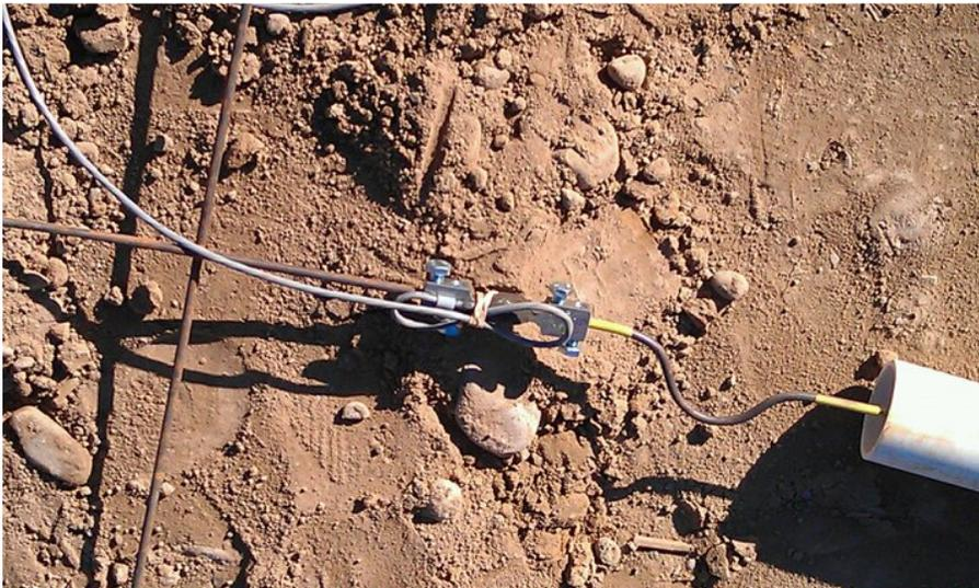
**Fig. 3.26.** Crimp showing yellow paint before construction (Jensen, 2013)
