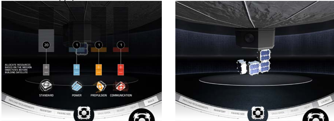
Figure 3. Screenshots of Beta version of an initial “app” for Satlet based design. The left image shows how various “resources” can be supplied to the satellite designer, and the right image shows how the graphical interface is able to “slide” satlets onto the screen, and rotate the image in 3D to “create” a new satellite around any payload.
