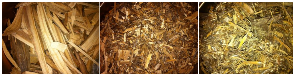
Fig. 2. 1. Photographs of various pinyon juniper fractions (a - PJ wood, b – PJ mixture, c – PJ bark)
