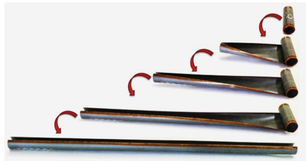
Figure 1: Example Fiber-Reinforced Polymer slit-tubes in various stages of deployment.
