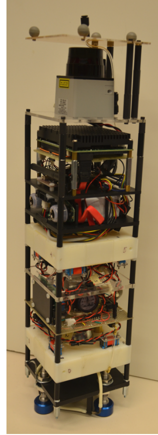
Fig. 2: The CubeSat Engineering Model with Components Related to Autonomous Proximity Navigation.
