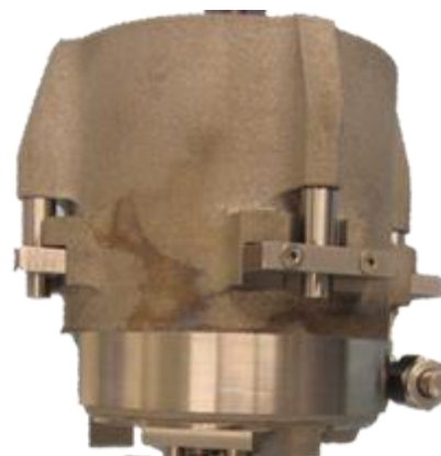
Figure 8: MPS-120 Piston tank system subassembly, with tooling attached for expulsion test purposes
