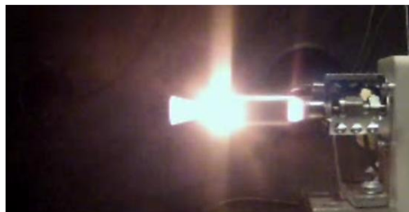
Figure 7: Busek’s 0.5N AF-M315E Thruster in Steady-State Firing at Full Throttle
