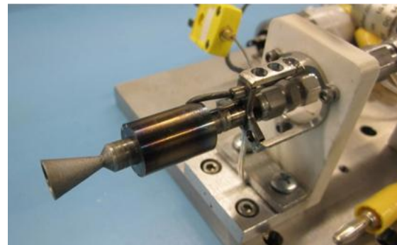
Figure 2: Post-Test View of a Fully Assembled 0.5N AF-M315E Thruster
