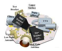
Figure 4 - Radiator Panel Equipment Layout Upper View
