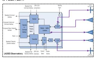
Figure 2 – LADEE S-Band Communications Subsystem Block Diagram
