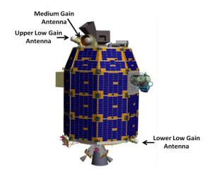
**Figure 6 - Antenna Mounting Locations**
