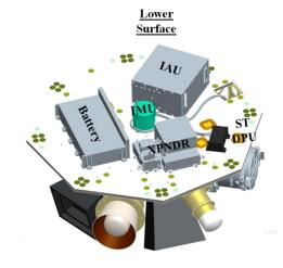
Figure 5 - Radiator Panel Equipment Layout Lower View
