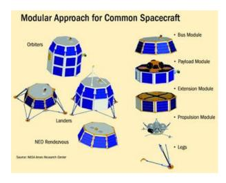
Figure 1 – Modular Approach for Common Spacecraft<sup>2</sup>
