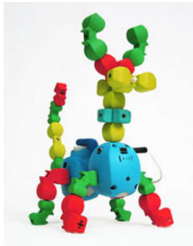
Figure 8. Topobo. ( http://www.topobo.com ). The large blue pieces are motors that can be programmed through motion. The yellow, green and red pieces attach to form a creature's structure.
