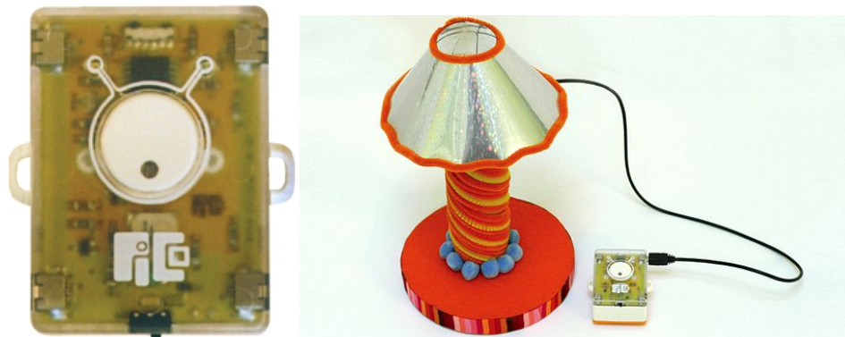
Figure 10. PicoCricket and an interactive lamp project using PicoCricket where the light changes colors based on sensor input.
