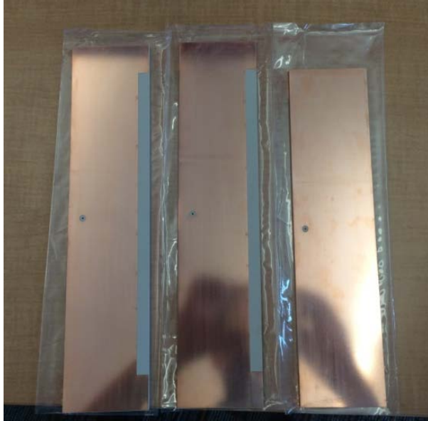
Figure 11. 434 MHz antennas. The left two show the PIFA designs with a notch, while the one on the right has no notch.
