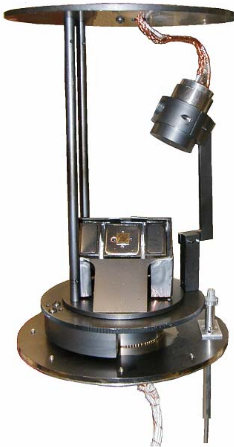
Figure 3- 1 The Chamber Apparatus contains a sample, two tertiary detectors, and a rotatable detector.
