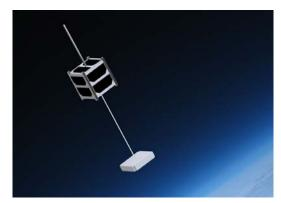
Figure 10: MiTEE Mission Spacecraft Concept Showing the CubeSat Deploying the Picosat
