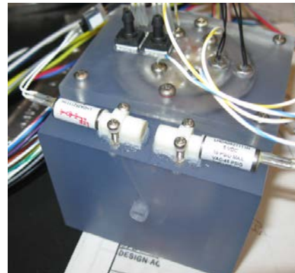
Figure 16 Photograph of a prototype thruster for initial thrust testing.
