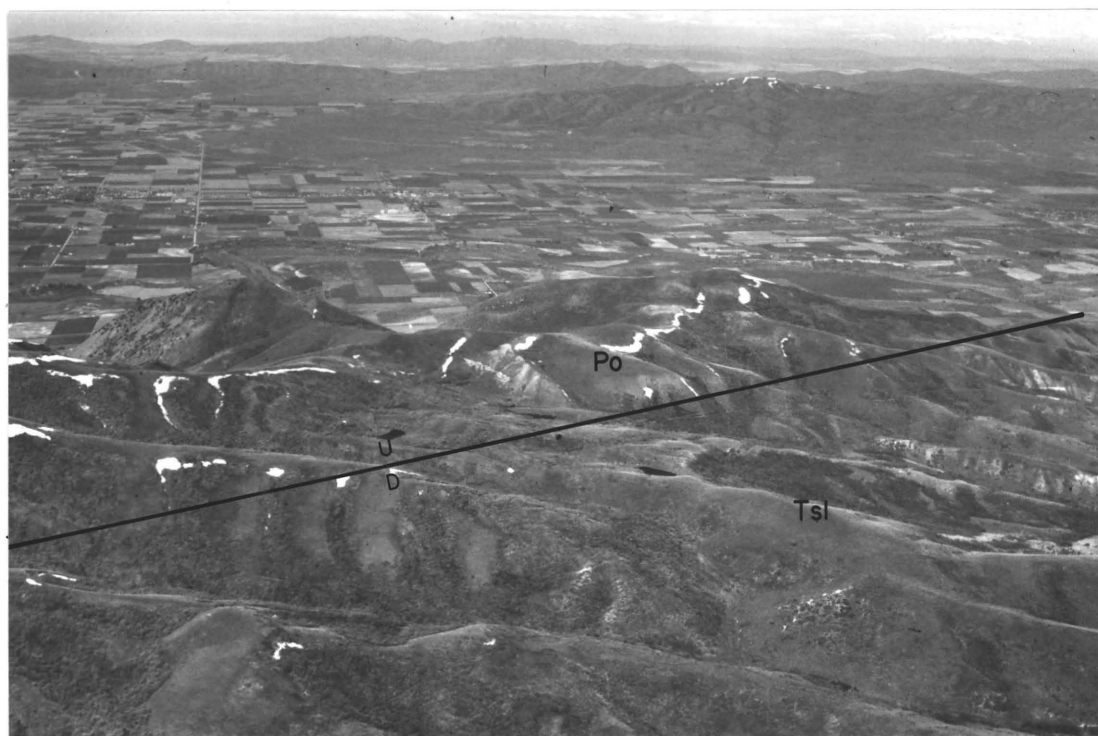
Figure 8. Normal fault in the northeastern part of Wellsville Mountains; aerial view west. The fault strikes N. 38^{\circ} W. and dips 80^{\circ} to 88^{\circ} E. It places the Salt Lake Formation (Tsl), on the northeast, down next to the Oquirrh Formation (Po). Refer to Figure 7.
