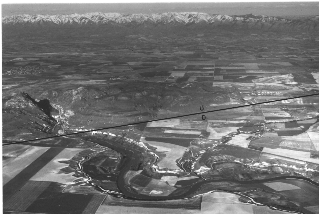
Figure 6. Normal fault along western side of Cache Butte Divide; aerial view east. The fault strikes N. 32^{\circ} W. and dips steeply west. It places the Oquirrh Formation, which underlies Lake Bonneville Group in the foreground, down relative to the Fish Haven-Laketown Formation, in Cache Butte Divide. The fault forms the northeastern boundary of a northwest-southeast-trending graben.
