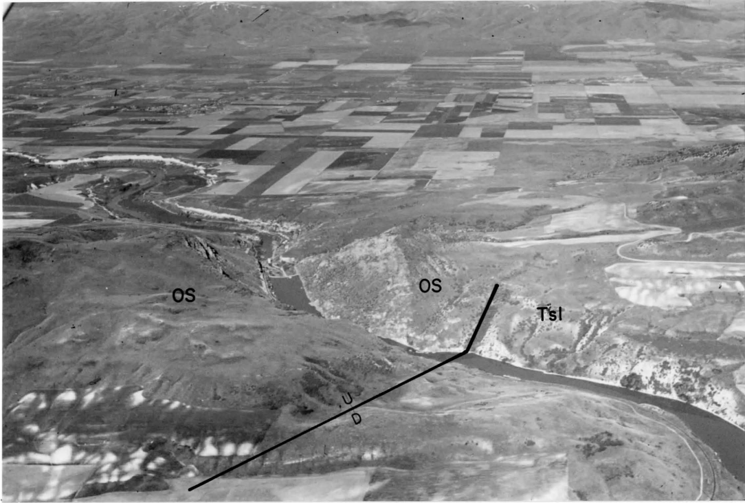
Figure 3. Normal fault in eastern part of Bear River Narrows; aerial view west. The fault strikes N. 72° W. and is vertical. North of Cutler Reservoir, the fault places the Salt Lake Formation (Tsl), on the north, down next to the Fish Haven-Laketown Formation (OS). South of the reservoir, the fault is obscured by the Lake Bonneville Group.
