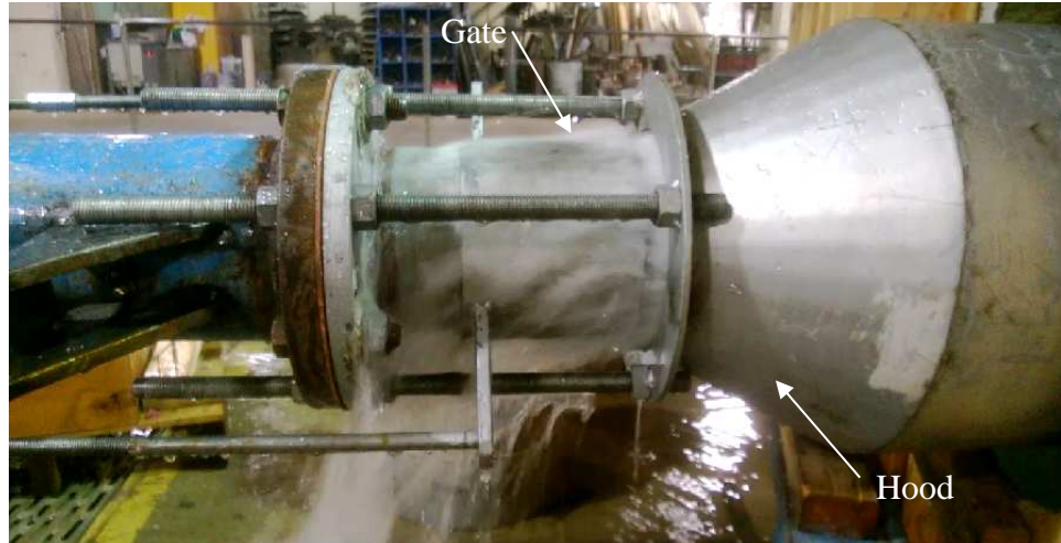
Fig. 2. Backsplash occurring with a hooded-FCV.
