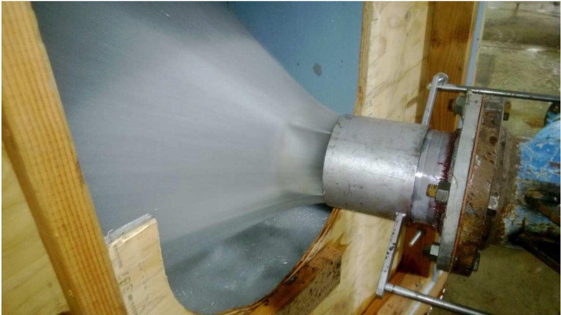
Fig. 6. Photo of conical jet of water.
