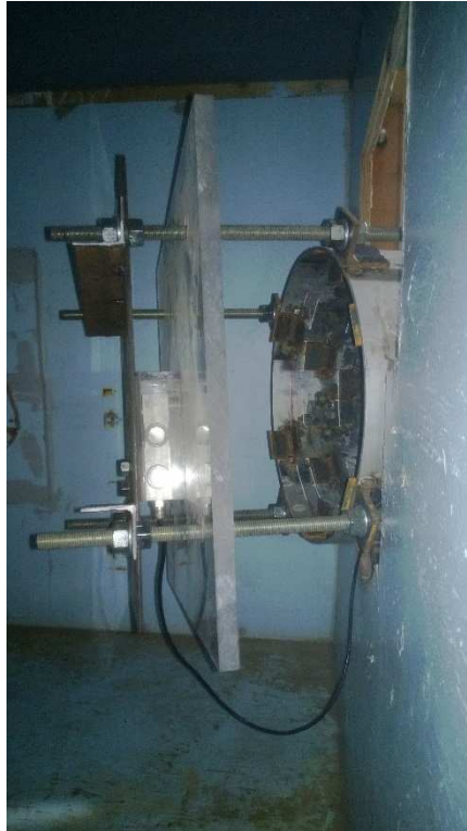
Fig. 11. Testing setup of downstream power measurement.
