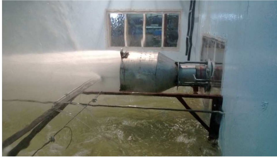
Fig. 9. Photo showing velocity measurements at free discharge.
