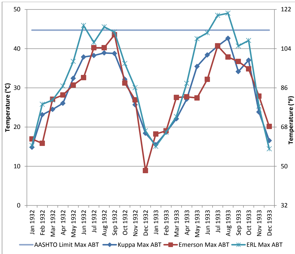
Figure 34. Monthly predicted maximum average bridge temperature for the California bridge (1932-1933).
